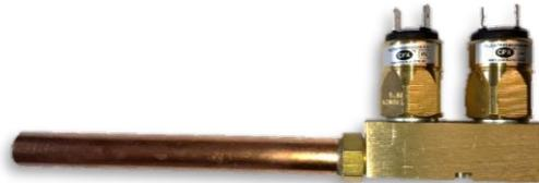
Each pressure switch shall be connected to the pipeline on a 100% gas tightness with removal Dowty bonded type seal, O-ring shall not be used to avoid blocking of pressure and creep. A brass block with twin 1/4" BSP port incorporating minimum leak to enable live change of pressure switch. Pipeline connection shall be a copper stub pipe to EN13348 and minimum leak brass 1/8" connection including Viton seal for 100% gas tightness.
